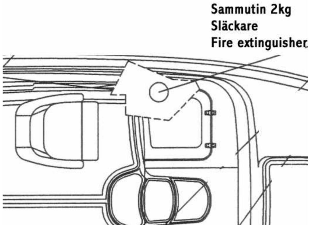
YAMARIN 59 Day Cruiser. Location and rating of portable fire extinguisher
