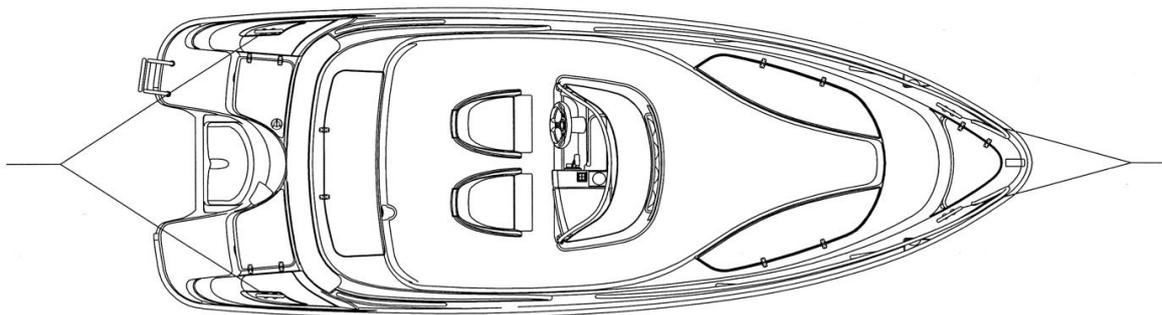
**WARNING!** When towing, the towline is under high tension. If it breaks, the speed of the end that has snapped off may rebound and cause serious injury or death. Always use a thick enough rope and do not get in the way of the rope extension.
