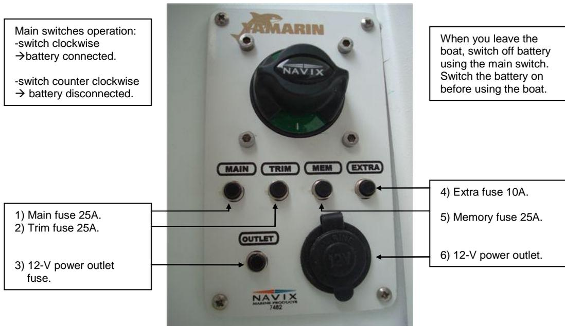
Fuses number one, two three, four and five are automatic. In case of short-circuit current automatic fuse will trigger itself. You can "prime" it again by pressing it back in. If the automatic fuse releases itself again you have a short-circuit in your electric system or in some component, in which case please do contact an authorised service shop.
