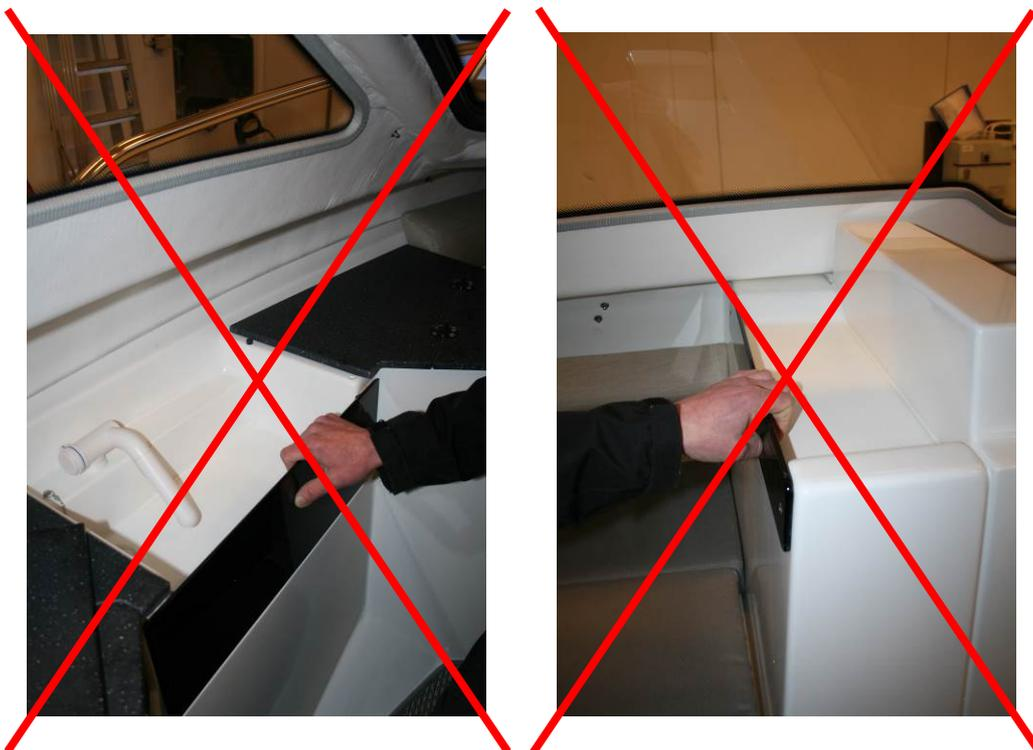
Image: The acrylic front edges in the cabin should not be used as handles.
