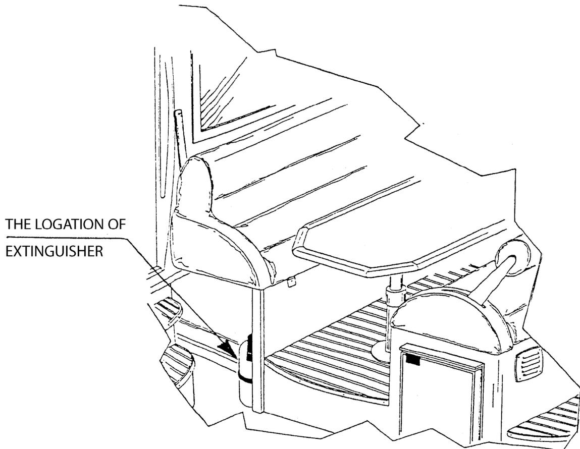
YAMARIN 74 Cabin. Location and rating of portable fire extinguisher
