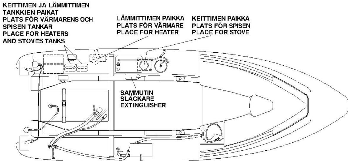
Yamarin 76 Day Cruiser location of portable fire extinguisher
