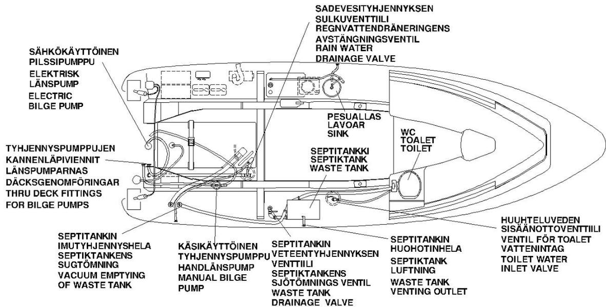
Yamarin 76 Day Cruiser locations of hull and deck thru fittings and closing valves.
