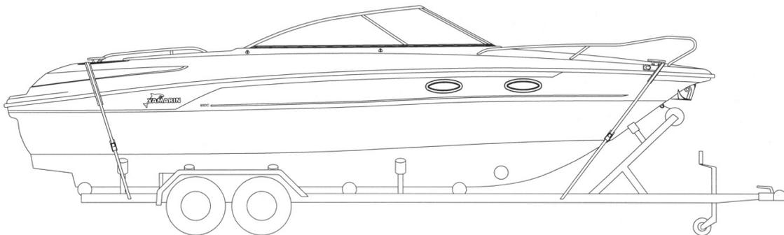
Image: Securing the boat to the trailer
