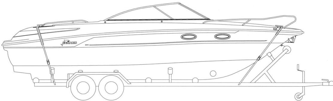
Tie the boat properly before starting the transport. Fastening belts located at the bow should be directed "down-back" and fastening belts located at rear should be directed "down-front". Do not leave any loose equipment or extra load to boat when it's transported. Take seat cushion away and close the hatches properly.
