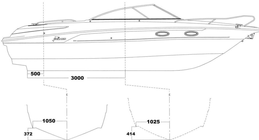
Only use reputable lifting companies or boat yards with sufficient lifting capacity. In addition to the boat's own weight (please refer to technical specification), also take into consideration the accessories and other possible loads on the boat.
