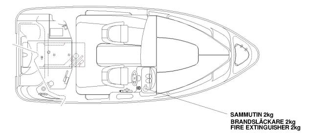
The portable fire extinguishers shall be serviced annually. Over ten years old extinguishers are not accepted without new pressure testing of the container. If you replace portable fire extinguishers, the new ones shall have at least identical fire-fighting capacity.
