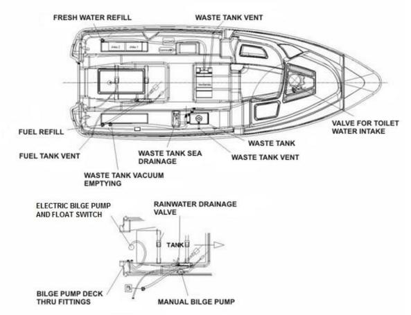
Locations of hull and deck thru fittings and closing valves for the Yamarin 68 Day Cruiser
