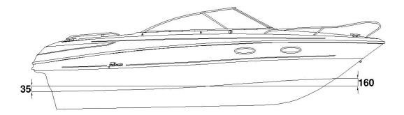
At stern:From chine 35 mm up with Yamaha F115, 50 mm up with Yamaha F250At bow:From chine 160 mm down
