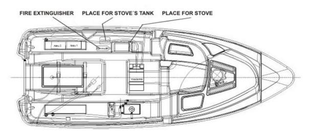
The location of the portable fire extinguisher on-board the Yamarin 68 Day Cruiser.
